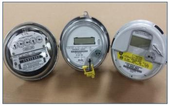
Consumers Energy has upgraded meter technology for residents and small businesses from electromechanical meters (left) to digital meters (middle) over the past 10 years, as the older meters have required replacement. Digital communicating meters (right) have upgraded functions and will be installed across the state through 2017.
